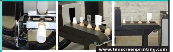
TMI Serpent UV dryers are designed for high speed drying of containers and 3D objects that require rotation to cure UV inks on a print surface that is not flat. Custom grippers on a heavy duty conveyor system easily and securely grasp the object, carrying it a short distance from the press to the drying chamber. As the object passes through the shielding into the chamber the gripper is automatically turned to allow complete exposure to the UV lamp and reflector system.
